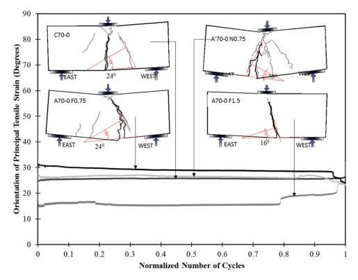
Fig. 8—Crack pattern and inclination of principal tensile strain (10M-70%Pu).
