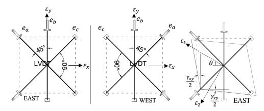
Fig. 3—LVDT strain transformation.
