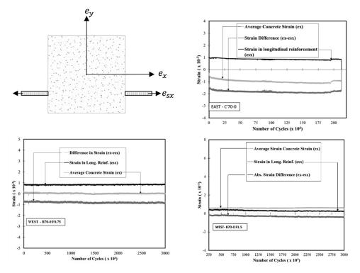
*Fig. 16—Evolution of concrete and reinforcement strain variation.*
