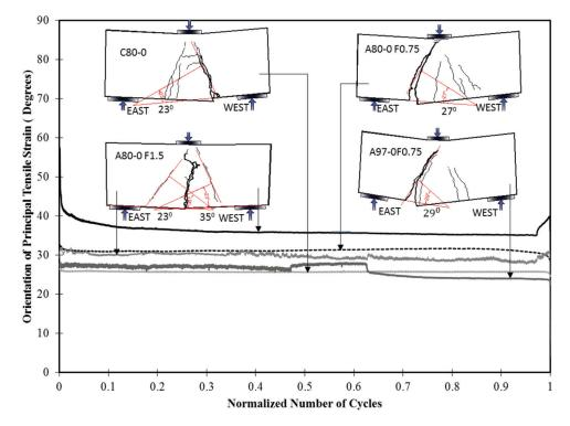
Fig. 7—Crack pattern and inclination of principal tensile strain (10M-80%Pu).
