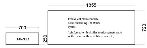
Fig. 17—Comparison between steel fiber-reinforced beam and conventional reinforced concrete beam. (Note: Dimensions are in mm; 1 mm = 0.0394 in.)
