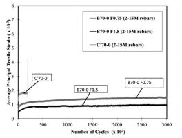
*Fig. 15—Average principal tensile strain evolution (2-15M).*
