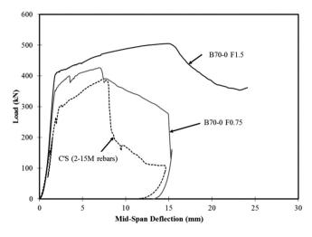
Fig. 5—Load-versus-deformation plot after fatigue loading.
