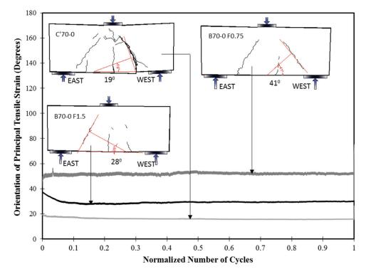
Fig. 6—Crack pattern and inclination of principal tensile strain (15M-70%Pu).
