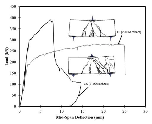
Fig. 2—Load-versus-deflection under monotonic loading (Beams C'S and CS). (Note: 1 kN = 0.225 kip.)
