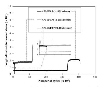
*Fig.* 4—Longitudinal reinforcement strain versus number of cycles at maximum load (2-10M reinforcing bars).
