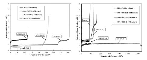
Fig. 13—Average shear strain evolution (2-10M).
