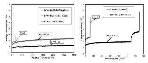
Fig. 10—Average shear strain evolution (2-15M).
