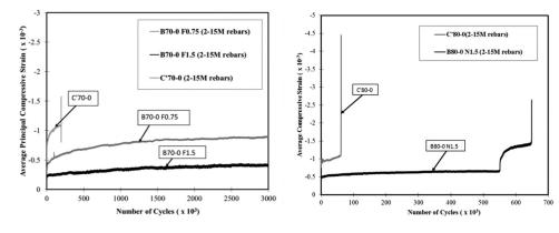
Fig. 14—Average principal compressive strain evolution (2-15M).
