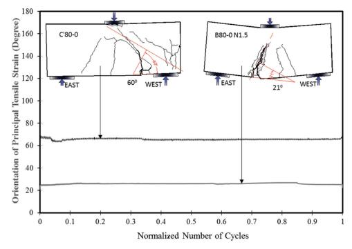
*Fig. 9—Crack pattern and inclination of principal tensile strain (15M-80%Pu).*
