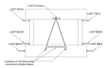
*Fig. 5—Instrumentation of wall.*
