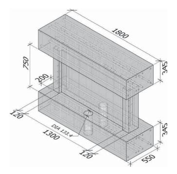
Fig. 1—Geometry of shear walls. (Note: All dimensions in mm;, 1 mm = 0.0394 in.)
