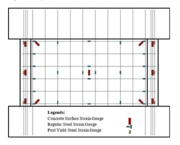
Fig. 3—Location of strain gauges.
