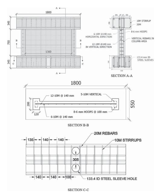
Fig. 2—Reinforcement details. (Note: All dimensions in mm; 1 mm = 0.0394 in.)
