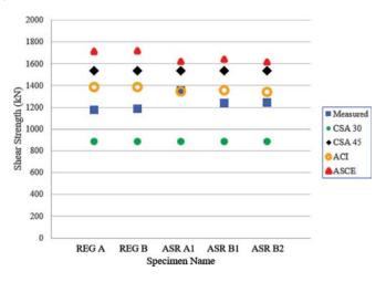
Fig. 10—Shear strength comparison between different codes and experiment. (Note: 1 kN = 0.225 kip.)
