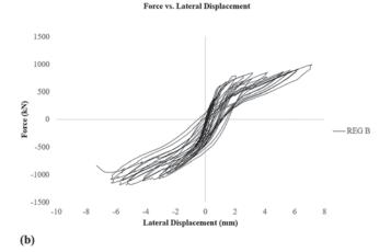
Fig. 7—Hysteresis responses of: (a) REG A; and (b) REG B shear walls. (Note: 1 kN = 0.225 kip; 1 mm = 0.0394 in.)
