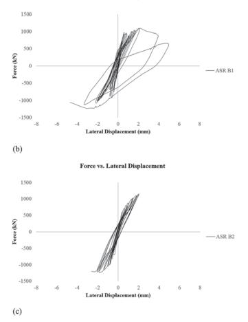
Fig. 8—Hysteresis responses of: (a) ASR A1; (b) ASR B1; and (c) ASR B2 shear walls. (Note: 1 kN = 0.225 kip; 1 mm = 0.0394 in.)
