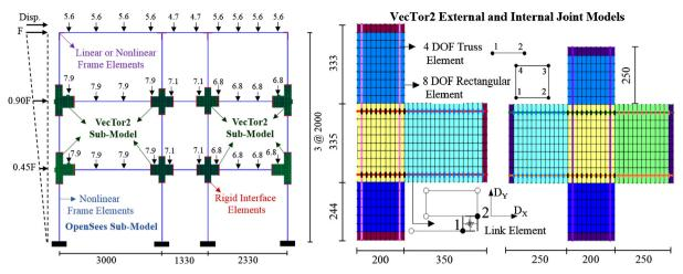
Fig. 6. Multi-platform model of RC frame with eight joints modelled with VecTor2 (dimensions in mm & forces in kN, 1 mm = 0.04 in., 1 kN = 0.225 kip).
