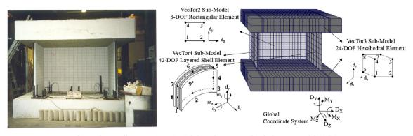
Fig. 3. Shear wall test specimen [36] (left) and Type B multi-platform FE model (right).
