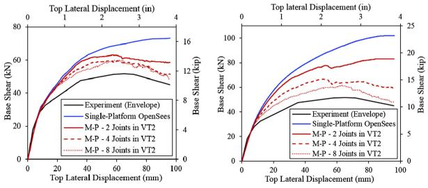
Fig. 7. Load-deflection responses of frame for push-over analyses of Type A models (left) and Type B models (right).
