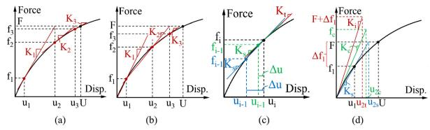
Fig. 1. (a) incremental tangent-based method; (b) incremental secant-based method; (c) approximation of secant method with tangent method; (d) combination of total solution methods.
