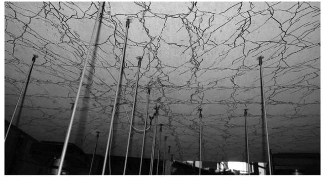
Fig. 9—R/FRC Slab TH5 after final impact, bottom surface.
