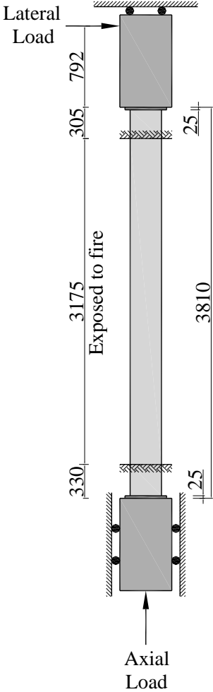
Figure 5-77 Mechanical and thermal loading setup of NRC Column 1582
