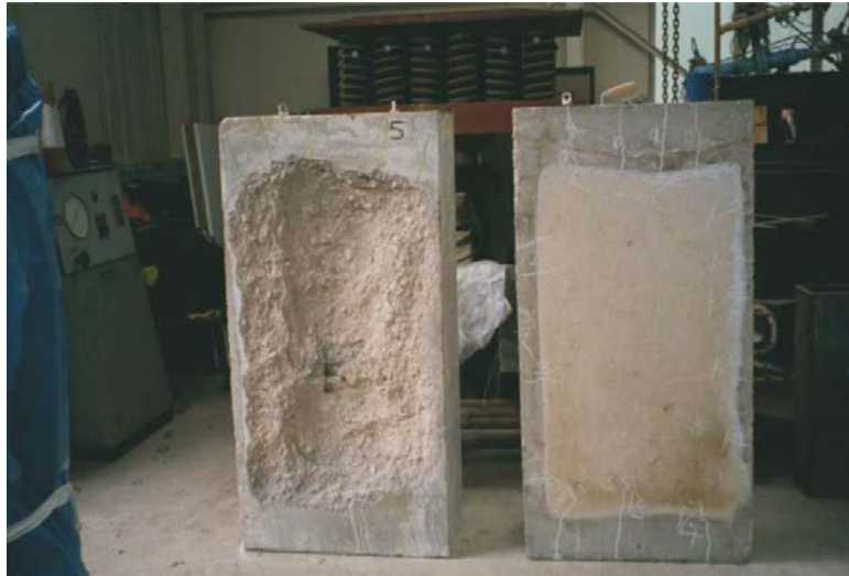
Figure 3-5 Spalling extent in HSC with (right) and without (left) polypropylene fibres (Shuttleworth, 1997)
