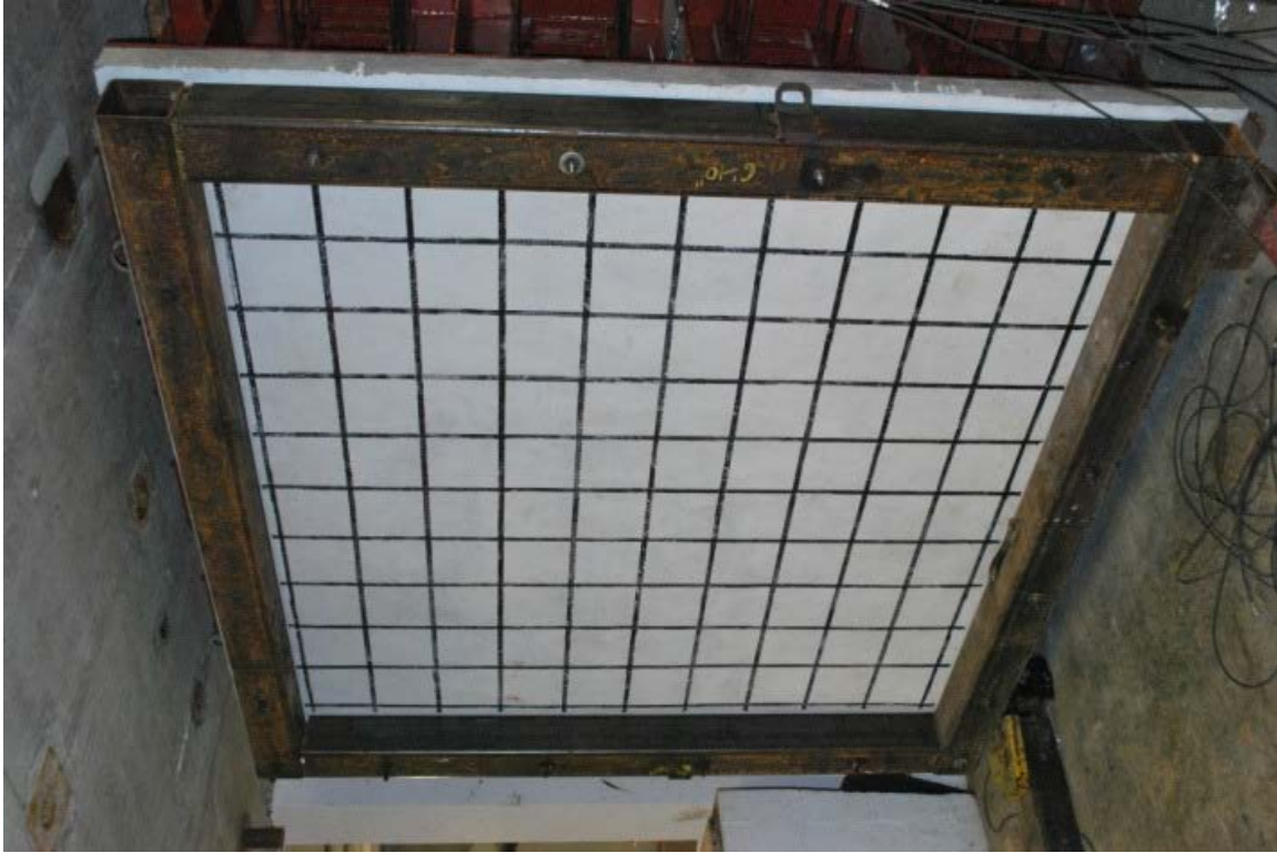
Figure 5-28 Fully-fixed support conditions of Jacques specimen CS5-C (Jacques, 2011)
