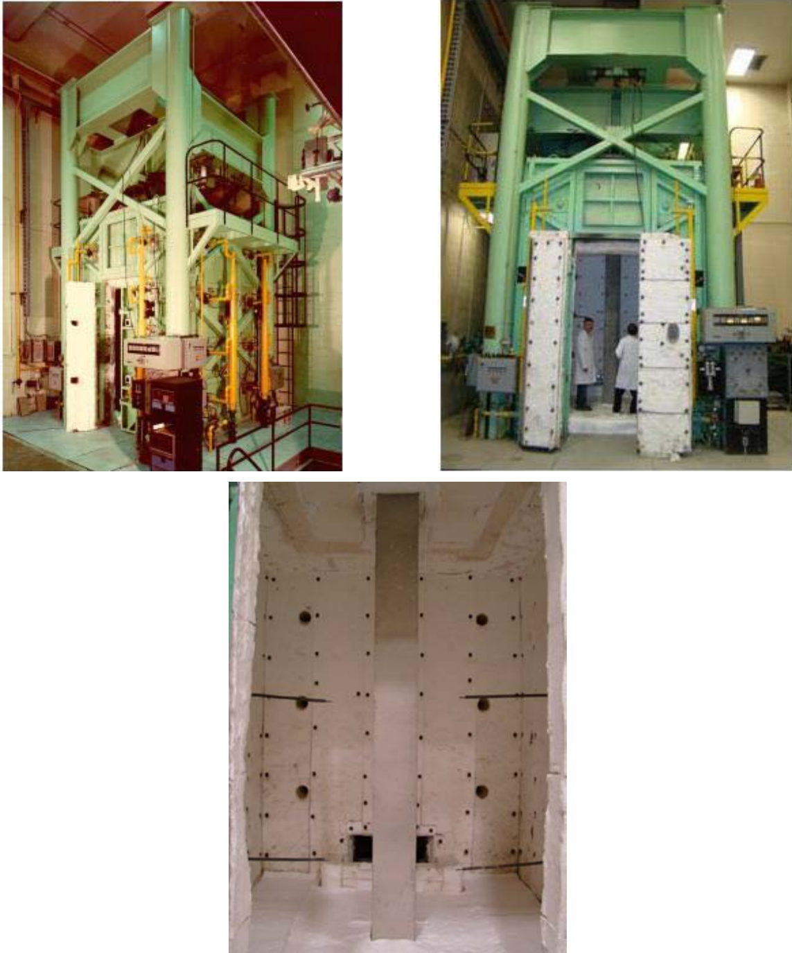
Figure 5-39 NRC Column Furnace Facility (Mostafaei et al., 2012)
