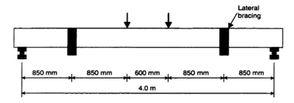
Figure 4-1 Test configuration for half-scale beams (Gentile, 2000)
