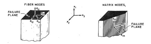
Figure 2-3 Failure modes and failure planes (Hashin, 1980)
