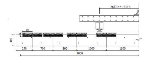
Figure 5-18 Arrangement of Specimen F1 (Yeoh, 2010)
