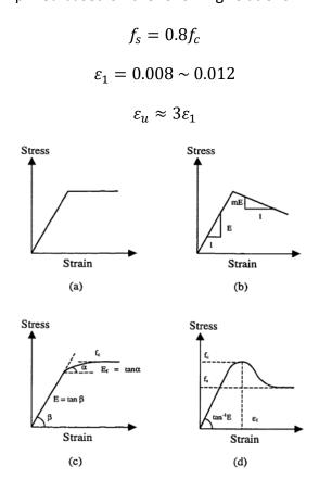
Figure 2-2 Proposed stress-strain curves in compression (Lau, 2000)
