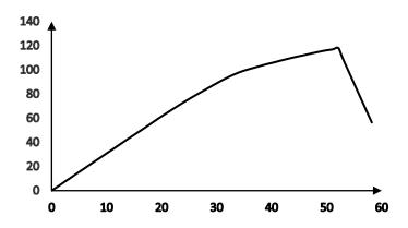
Figure 2-5 Typical load-deflection response of TCC
