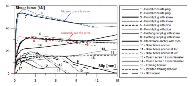
Figure 5-23 Adopted and adjusted load-slip curve (Deam et al., 2008)
