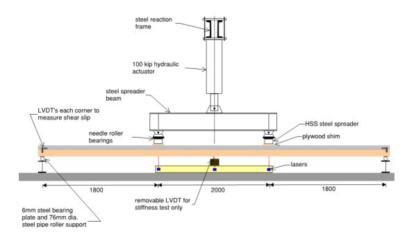
Figure 5-27 Experimental setup for Gerber Specimen
