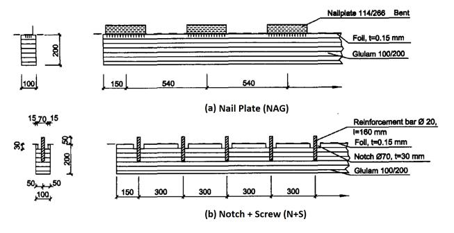
Figure 5-32 Connector Types (van der Linden, 1999)
