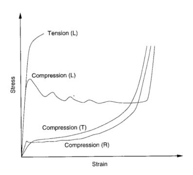
Figure 2-1 Typical stress-strain curves for wood (Holmberg et al.,1998)
