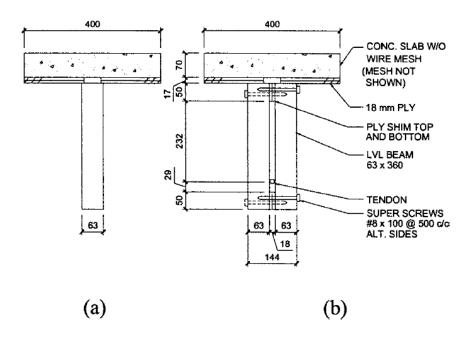
Figure 5-20 Cross sections of (a) CS1 and (b) CS3 (Deam et al., 2008)
