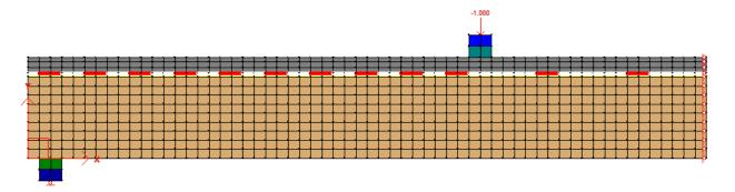
Figure 9 Completed FE model for Specimen CS1
