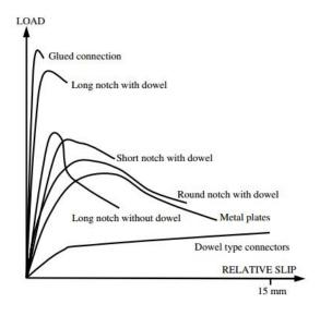
Figure 2-6 Comparison of different connection systems (Dias, 2005)
