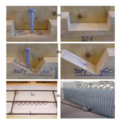
Figure 5-12 Variations of connections with and without coach screws: (a) rectangular; (b) triangular; and (c) toothed plate connection (Yeoh, 2010)
