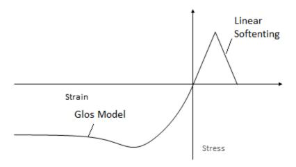
Figure 3-2 Typical stress-strain curve for wood (grain direction)
