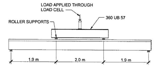
Figure 5-21 Test setup (Deam et al., 2008)
