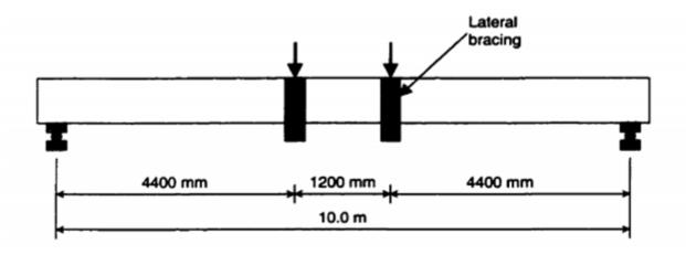
Figure 4-3 Test configuration for full-scale beams (Gentile, 2000)
