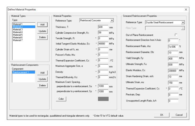
Figure 5-3 Concrete definition interface
