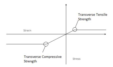
Figure 3-3 Typical stress-strain curve for wood (transverse direction)
