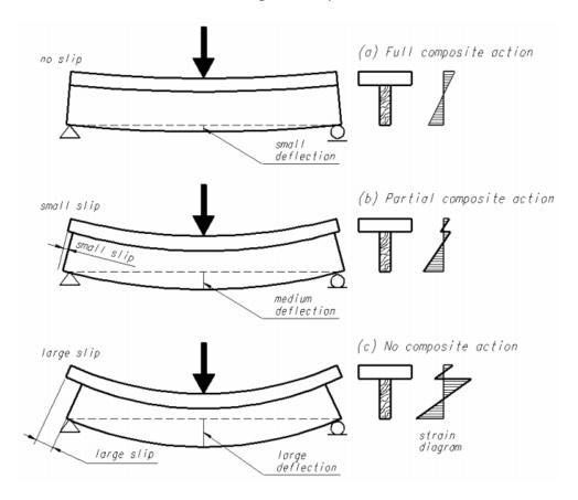
Figure 2-4 Definition of composite action (Lukaszewka, 2009)
