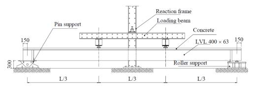
Figure 5-13 Typical four-point bending test setup (dimensions in mm) (Yeoh, 2010)
