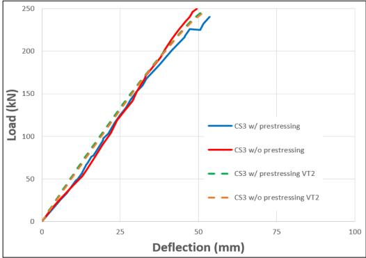
Figure 5-26 Load-deflection plots for Specimen CS1 and CS3
