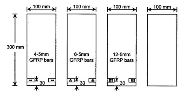
Figure 4-2 Cross sections of half-scale reinforced beams (Gentile, 2000)
