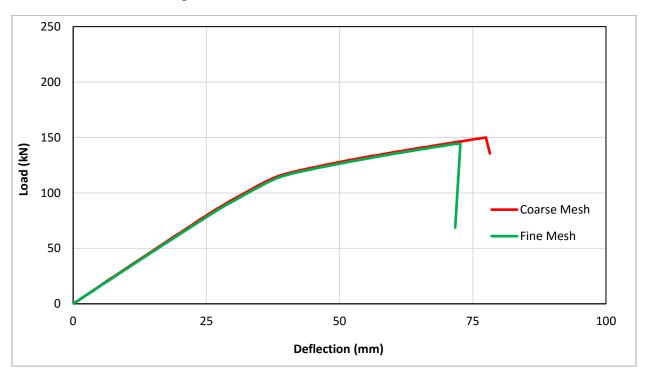
Figure 5-41 Comparison of predicted load-deflection responses of different mesh size
