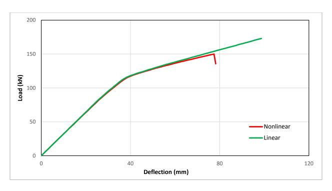
Figure 5-42 Load-deflection responses of Specimen CS1 with linear and nonlinear material constitutive models
