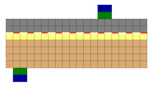
Figure 5-2 Sample model with discrete shear connectors
