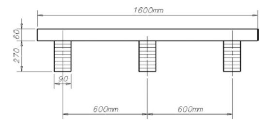
Figure 5-36 Specimen cross section (Lukaszewska, 2009)
