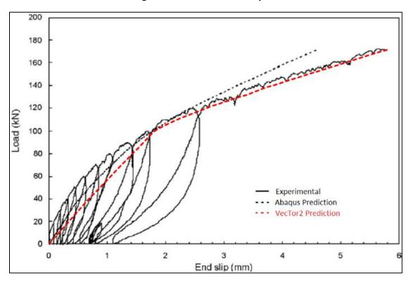
Figure 5-10 Load-slip plot
