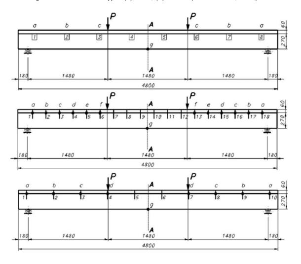
Figure 5-38 Connector Layout (a) Top: Specimen 1 and 5 (SP + N); (b) Middle: Specimen 2 and 4 (SST + S); (c) Bottom: Specimen 3 (SST + S) (Lukaszewska, 2009)
