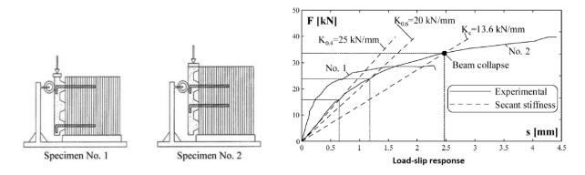
Figure 5-19 Specimen details and result (Cecotti et al., 2006)
