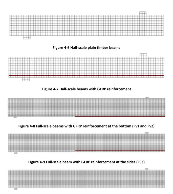
Figure 4-10 Full-scale plain timber beam (FS4)
