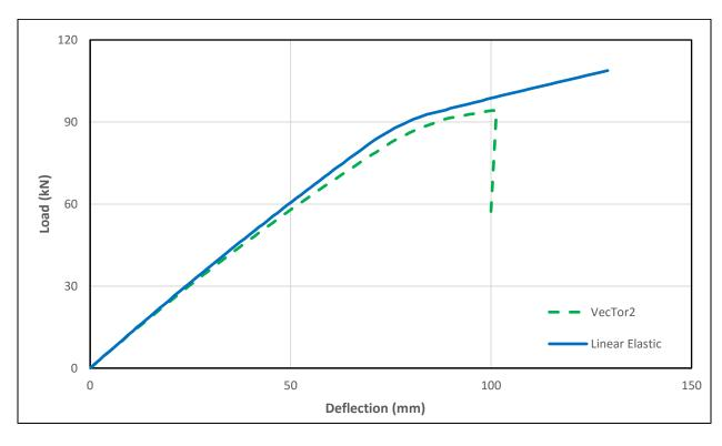
Figure 5-43 Load-deflection responses of Specimen S7 with linear and nonlinear material constitutive models
