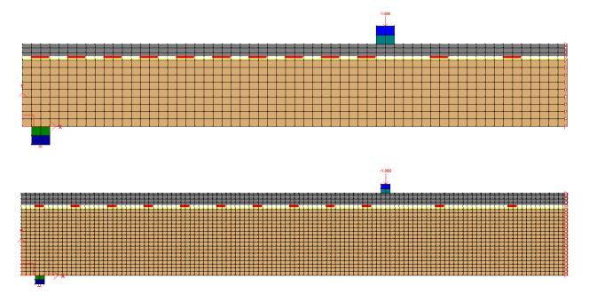
Figure 5-40 FE models with different mesh size
