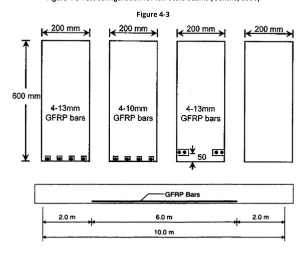
Figure 4-4 Configuration of full-scale reinforced beams (Gentile, 2000)
