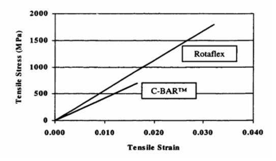
Figure 4-5 Stress-strain relationships for GFRP (Gentile, 2000)
