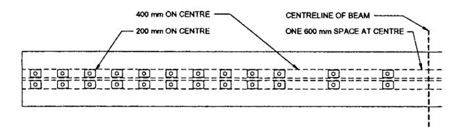
Figure 5-22 Connector layout for Specimen CS3 (Deam et al., 2008)
