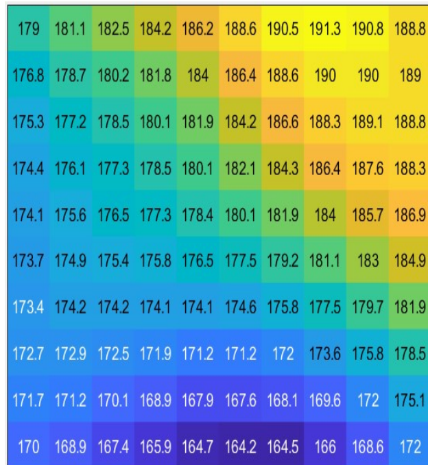
Figure 3.9: One random field generation of concrete compressive strength, f'_c .
